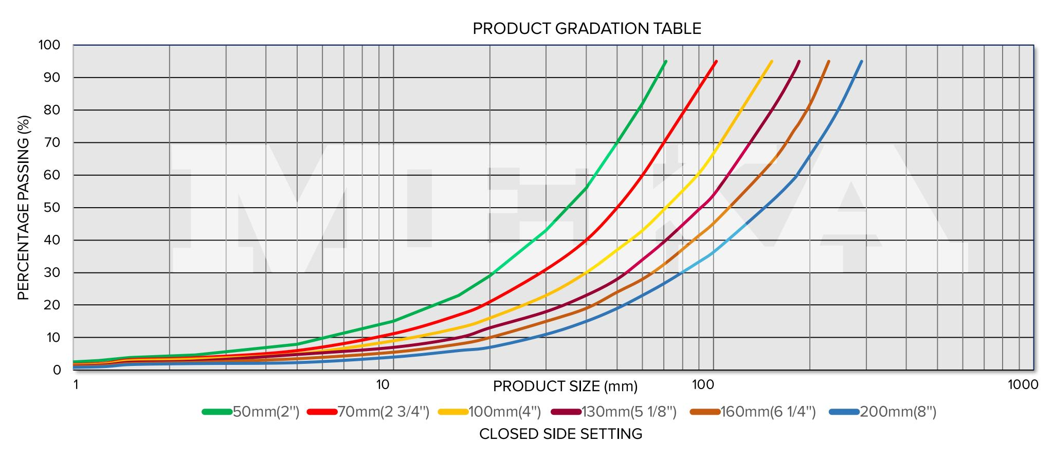
Results may vary depending on feed material gradation, density, moisture content, friability and crushing application.
