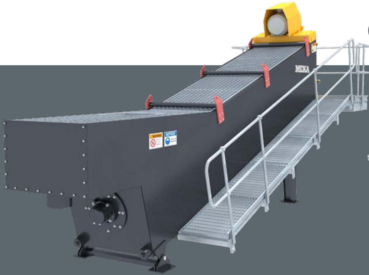
Coarse material washers are used to remove a limited amount of dirty material from a coarse aggregate. This material includes very water soluble slimes, silts, soft clay, and organic particles. They are often used as a final wash following a wet screen and are designed to scrub and clean gravel and crushed stone up to 75mm (3") in size. Both single and double spiral units are available depending on the capacity required.
