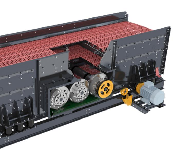
Proven oval stroke design increases production, reduces recirculation load. Oval throw action makes MEKA screens virtually non-plugging and raises quality output. The ability to fine tune stroke angle, amplitude and speed adds versatility in meeting changing screening conditions. Extra-strong body construction, durable bearing mountings, computer designed chrome-moly-nickel gear set with premium metallurgy extend service life.
