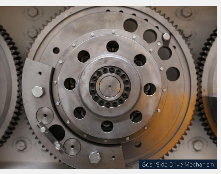
Adjusting the stroke angle has been found to be the most influential in optimising the screen efficiency. Higher stroke angles increase the number of chances the material has to pass through the openings and also increases the impact to shake fines loose. Lowering the stroke angle increases the travel rate for heavy screening or scalping operations. Higher speed is sometimes desired for scalping duty.
