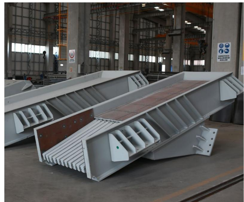
Pan feeders with grizzly scalper are utilized in the primary. The separate scalper unit offers very good separations optimized for effective scalping and fines removal. A long stroke capability means better scalping efficiency, delivering a linear motion with high G force (5.5 G).
