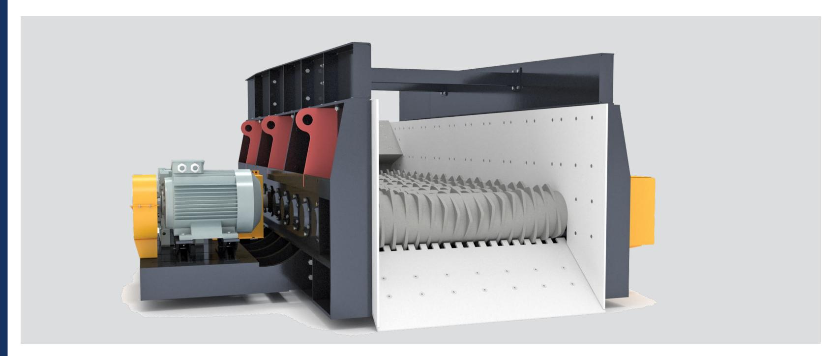
Exclusively designed non clogging and self cleaning elliptical bars, it is a sturdy machine suitable for heavy duty work. Recommended for pre-screening and cleaning of dirty material with a high content of clay and moisture.
