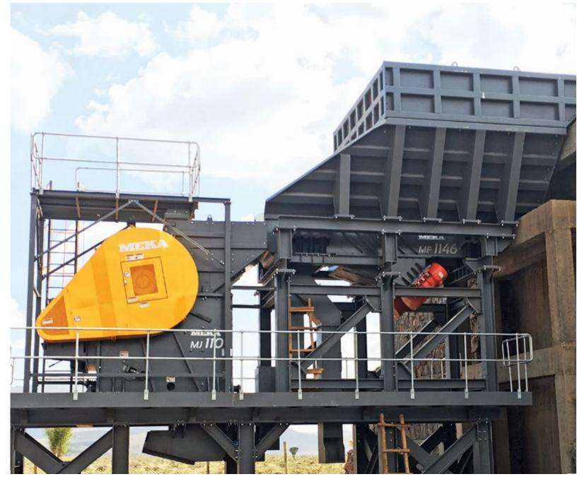
The heavy duty design of the feeder pays off in open pit applications with coarse feed of up to 1000 mm to match large jaw crushers and primary impact crushers.
