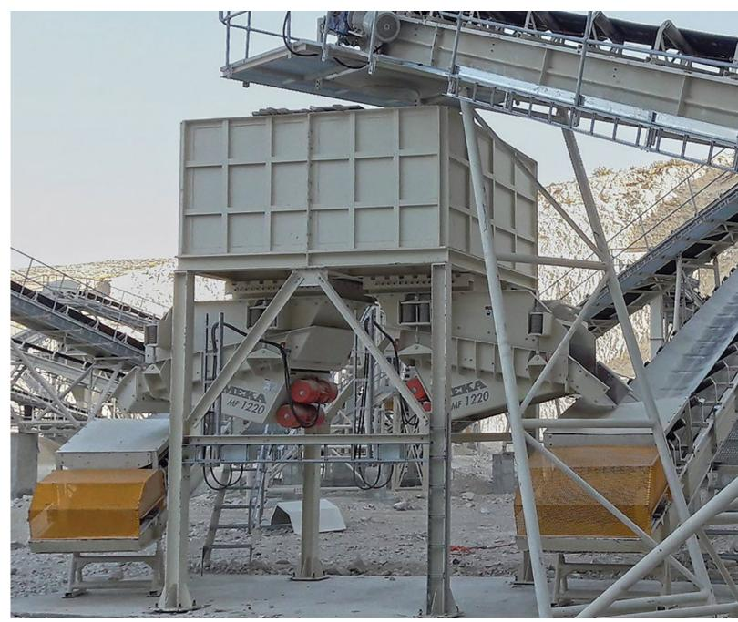
The high capacity vibrator motors generate up to 10mm stroke for maximum production in most any materials from small granular materials to large lumps produced from primary crushers.
