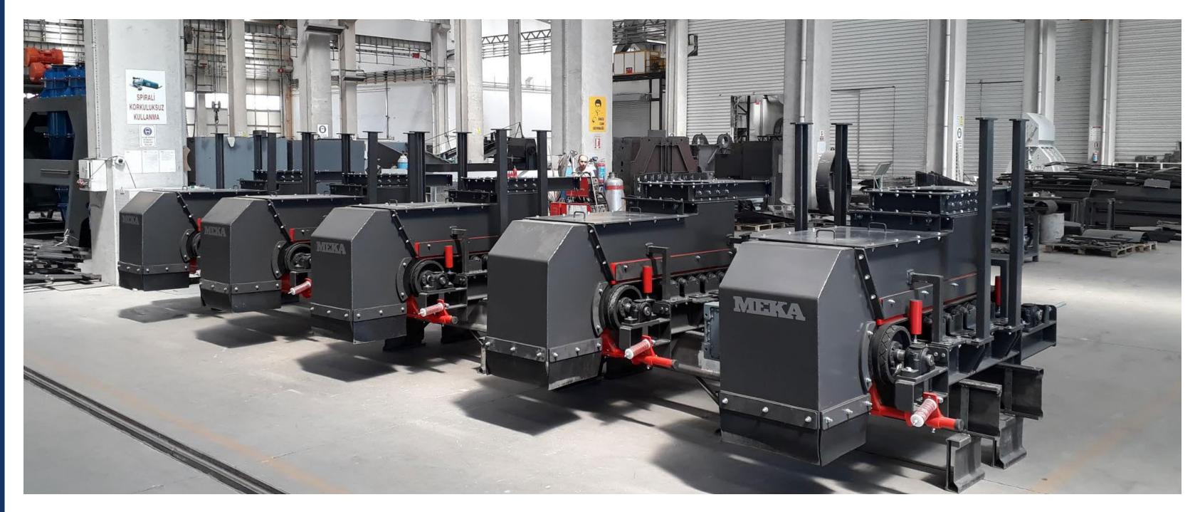
Belt feeders are short belt conveyors that are specifically designed for material flow regulation, extracting material from one area and ensuring that downstream equipment receives the appropriate volume.
