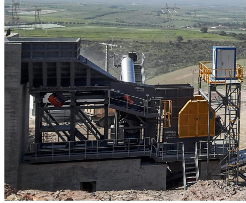
The separate scalper unit offers very good separations the stroke length, stroke angle and motor speed can be optimized for effective scalping and fines removal. A long stroke capability means better scalping efficiency, delivering a linear motion with high G force (4.5 G).
