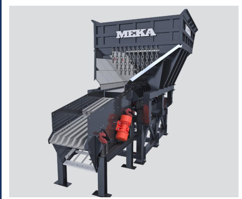
Pan feeders with grizzly scalper are utilized in the primary crushing stage, typically when excessive clay or an abun-since it runs independently of the feeder. Consequently, dance of fines are present. They scalp the primary feed allowing fines to bypass the primary crusher. Screening the fines before the crusher results in higher overall capacity of the primary crushing stage
