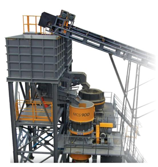
This type of cone crusher is suitable for high-capacity secondary crushing applications where a larger feed opening is required. Crusher has a larger intake capability and a high capacity in relation to its size.
