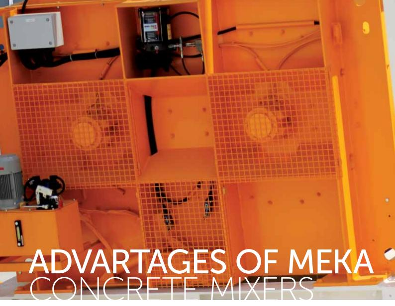
**Heavy and Robust:** MEKA Twin-Shaft concrete mixers offer long life, as they are 5-10% heavier than most of their equivalents on the market today, due to their robust steel structure and thick interior abrasion proof linings.
