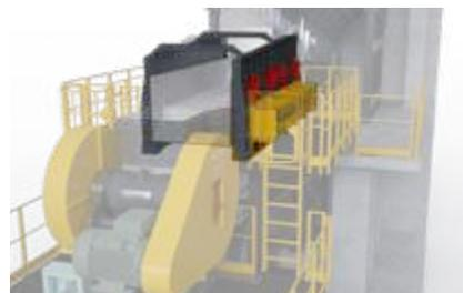
Wobbler feeders are the most suitable feeder type for feeding and screening all kinds of moist, sticky ores and rocks in mining and quarry applications.
