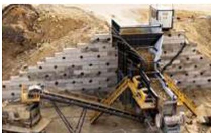
Other types of feeders and screens may have problems such as plastering and clogging in wet and sticky materials, Wobbler feeders are suitable for these types of materials.
