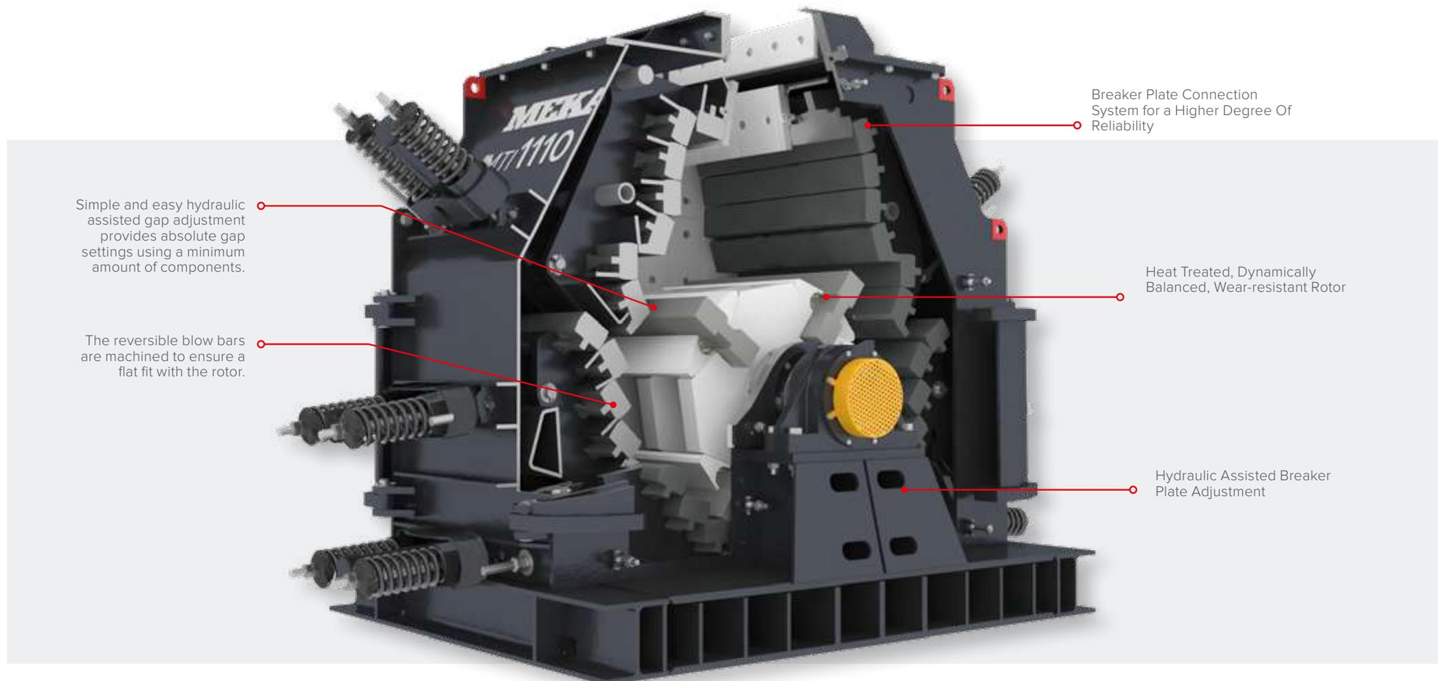
Breaker Plate Connection System for a Higher Degree Of Reliability
