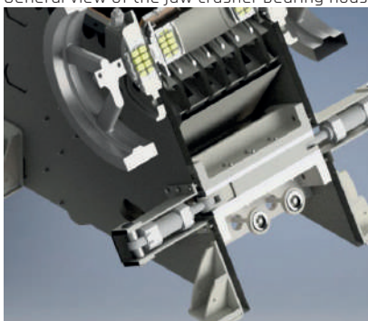
Double-toggle hydraulic jaw adjustment system.
