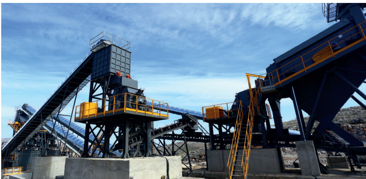
Feeding of MEKA Tertiary Impact Crusher with a Vibrating Feeder
