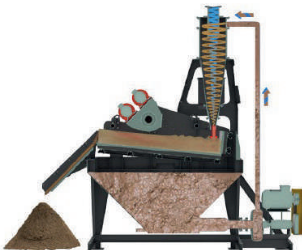
MEKA Compact Sand Unit Working Principle
